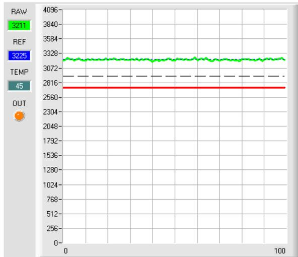
As long as the current measurement value **RAW** (green line) lies above the switching threshold (red line), the output **DIGITAL OUT** is at +24V (signal is OK). This is visualised by the **OUT LED**.
