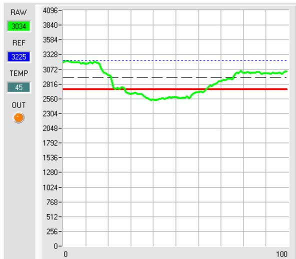
When the current measurement value **RAW** (green line) rises above the hysteresis threshold (black line) again, the output **DIGITAL OUT** changes to +24V again (signal is OK). This is visualised by the **OUT LED**.
